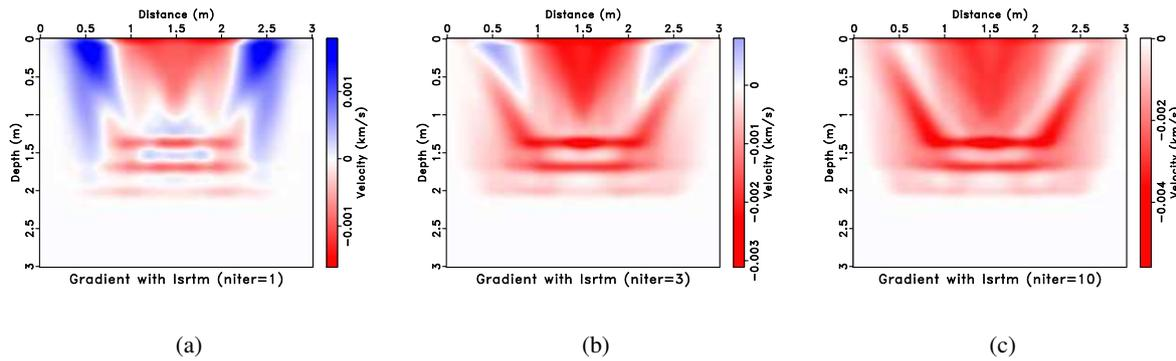
**Figure 2** Background velocity gradient using extended reflectivity image by linearized inversion after different iteration number (a) iteration 1; (b) iteration 3; (c) iteration 10.
