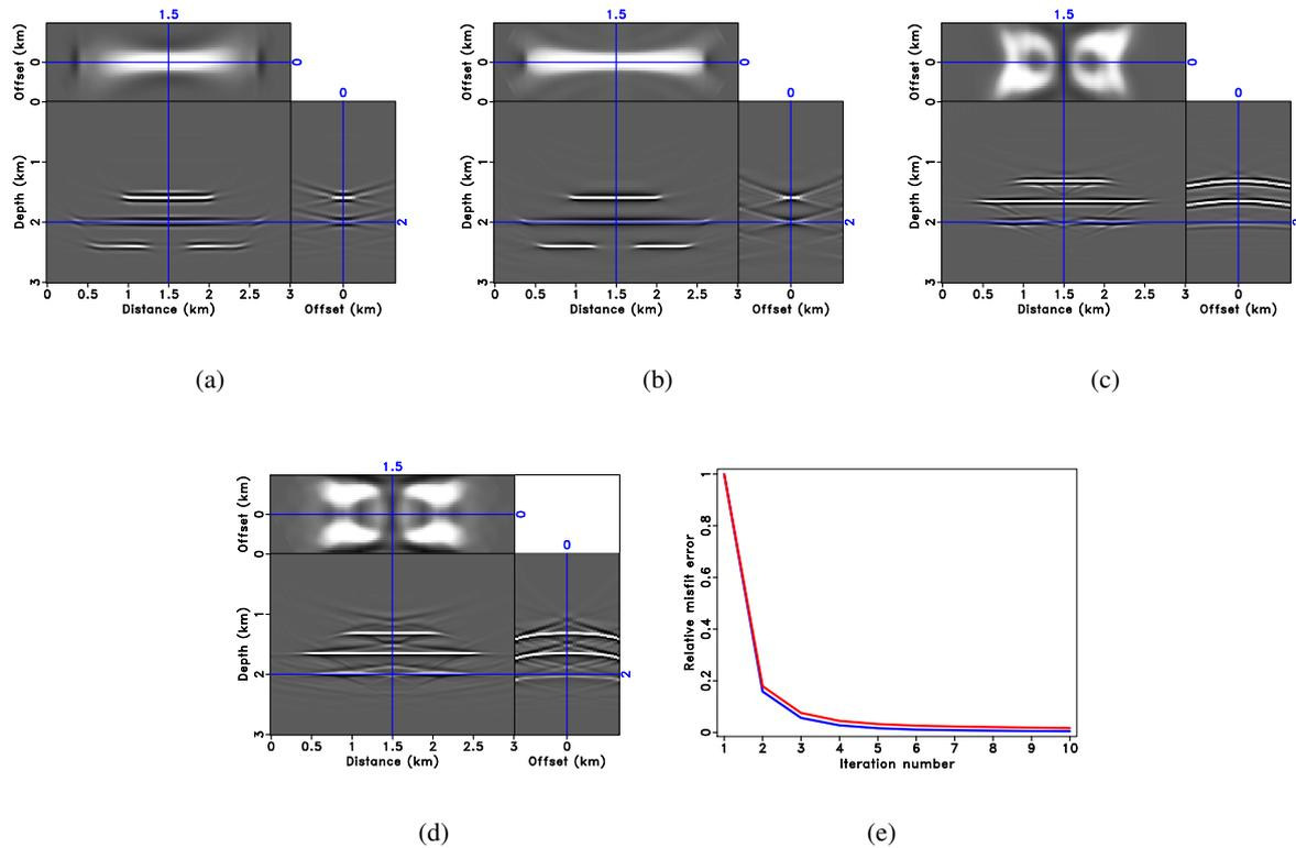
**Figure 1** Image of extended reflectivity (a) ERTM with correct velocity; (b) LSERTM with correct velocity after 10 iterations; (c) ERTM with wrong velocity; (d) LSERTM with wrong velocity after 10 iterations; (e) Relative misfit error of LSERTM with correct (blue line) and wrong (red line) velocity.
